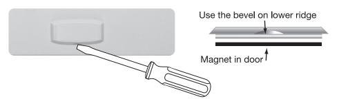
Gently slide a screwdriver into the bottom edge of the badge. Gently turn the screwdriver counter clockwise. The badge is held on by a magnet in the well of the battery door. The badge should pry off easily.
