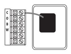
Remove factory battery tab when installing thermostat.
