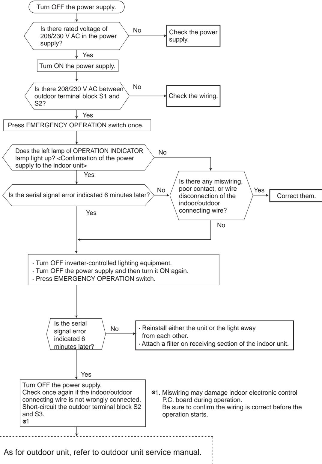
\*1. Miswiring may damage indoor electronic control P.C. board during operation.
