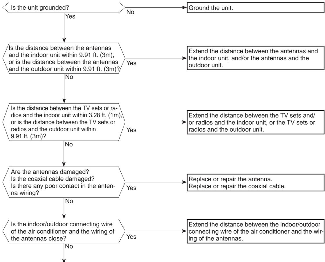
Even if all of the above conditions are fulfilled, the electromagnetic noise may enter, depending on the electric field strength or the installation condition (combination of specific conditions such as antennas or wiring).
