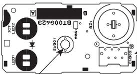
CN302 Indoor electronic control P.C. board connector
