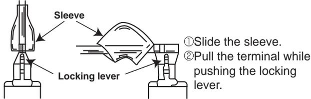
(2) The terminal with the connector shown below locking mechanism.
