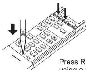
Press RESET button gently using a thin instrument.
