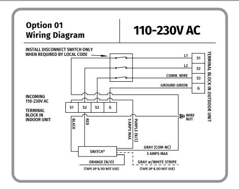
\*NOTE: Switch relays are shown with power applied to device.
