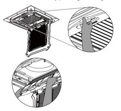
Remove the photocatalyst Deodorization filter by pulling upward.
