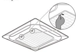
Remove PM1.0 filter by pressing the fixing hook.
