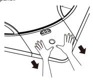
Open the PM1.0 sensor case on the side of the PM1.0 Sensor case and remove the rubber cap.
