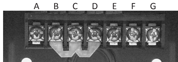
Fig. 3 Load / AC Input Connectors Terminal Block Model 9045
